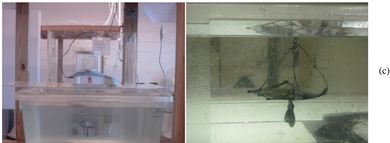
Figure 4. (c) Determination of shell weight of Isognomon alatus by buoyant weighing technique.
