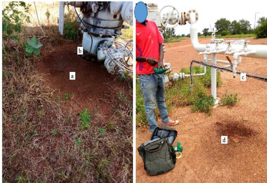
Plate 1. Oil spill at Croisement Ridina. (b)Well-near sampling points, (a), (c) and (d) drain points.
